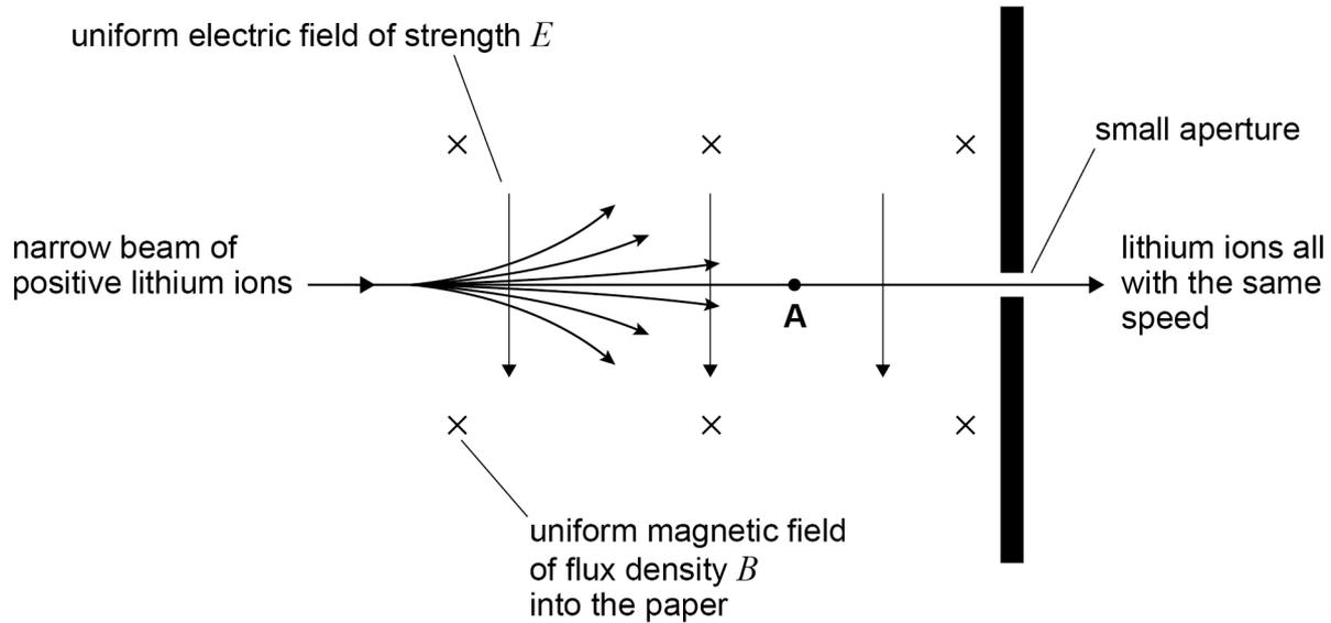
A narrow beam consists of positive lithium ions travelling at different speeds. The beam enters a region where there is an electric field and a magnetic field. The directions of the uniform electric field of strength  $E$  and the uniform magnetic field of flux density  $B$  are shown on **Figure 3**.
