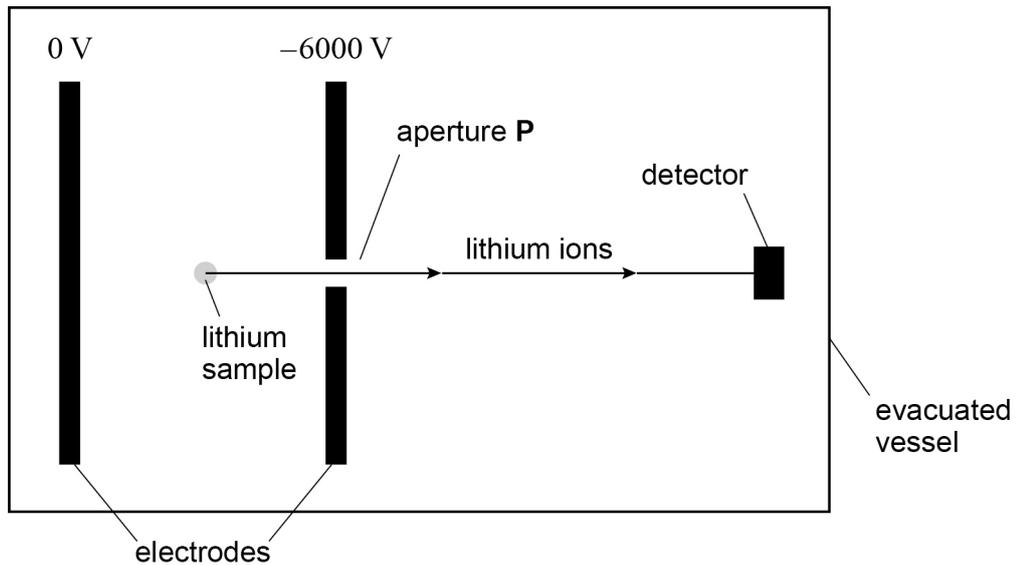
A stationary  ${}^7_3\text{Li}^+$  ion in the lithium sample is at the mid-point between the parallel electrodes. The  ${}^7_3\text{Li}^+$  ion accelerates towards aperture P.
